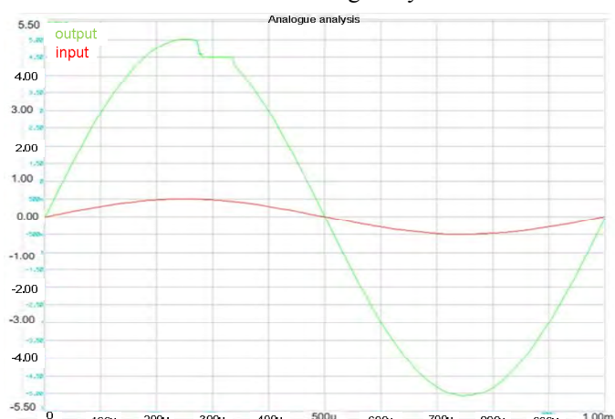
fig.2.1. Define the maximum amplification of the audio stage
