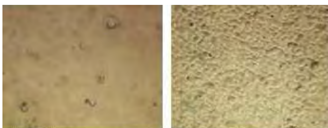
Fig. 8 PVDF layers sprayed at 80 °C and increased concentration on glass substrate, showing good adhesion, but low planarity and uniformity.
