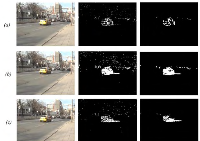
Fig. 2. Original image, foreground image and filtered foreground image executed for three values of T , T = 0.05 (a); T = 0.3 (b); T = 0.55 (c)
