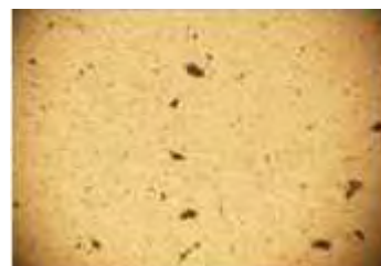
Fig. 2 PVDF layers sprayed at 20°C on glass substrate.
