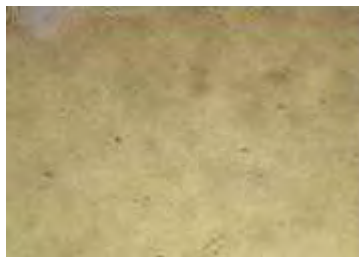
Fig. 7 PVDF layers sprayed at 100 °C on glass substrate, showing good adhesion, but low planarity and uniformity.
