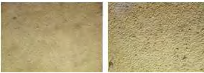
Fig. 6 PVDF layers sprayed at 80 °C on glass substrate (in left) and silicon substrate (in right), having higher adhesive strength.
