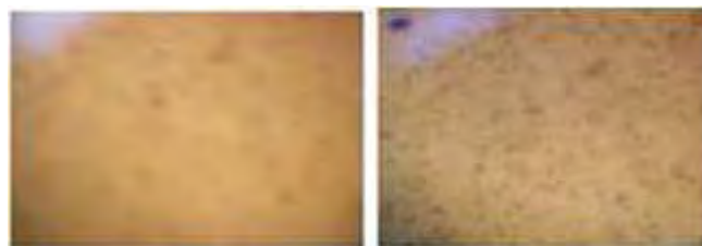
Fig. 3 PVDF layers after thermal treatment at 180°C.
