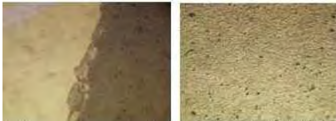
Fig. 5 PVDF layers sprayed at 70 °C on glass substrate (in left) and silicon substrate (in right), having lower adhesive strength.
