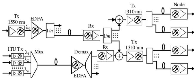
Fig. 2. Forward path configuration 2
