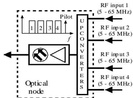
Fig. 3. Block conversion at an optical node
