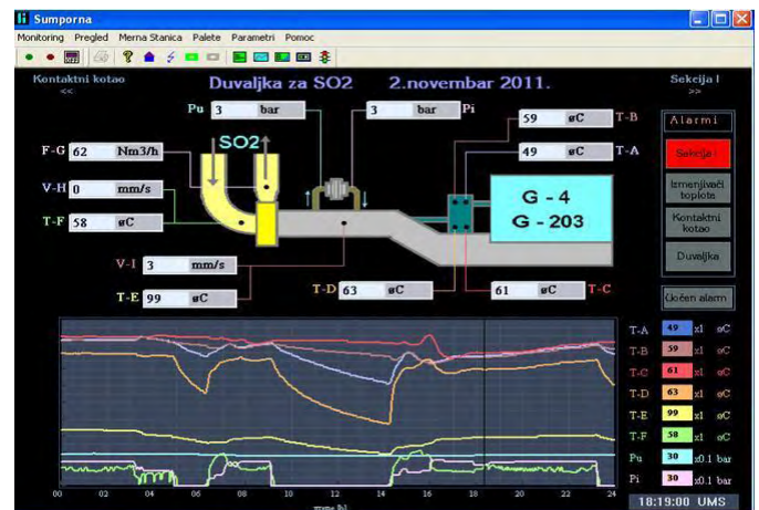
Fig. 5. Synoptic screen for the blower in the sulfuric acid plant
