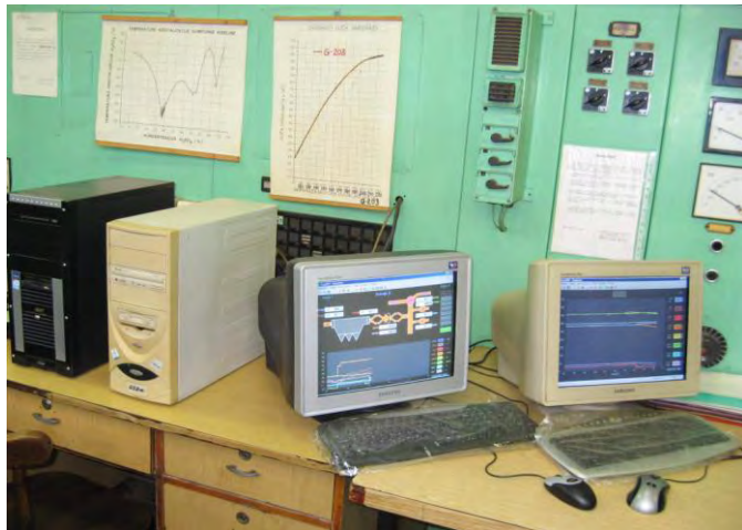
Fig. 7. Workstation with the RCP client running (left), side by side with server executing the PCP (right)
