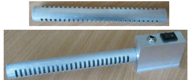
Fig. 3. Realized shotgun microphone prototype (the interference tube (above) and the whole microphone of length of 242 mm (below))
