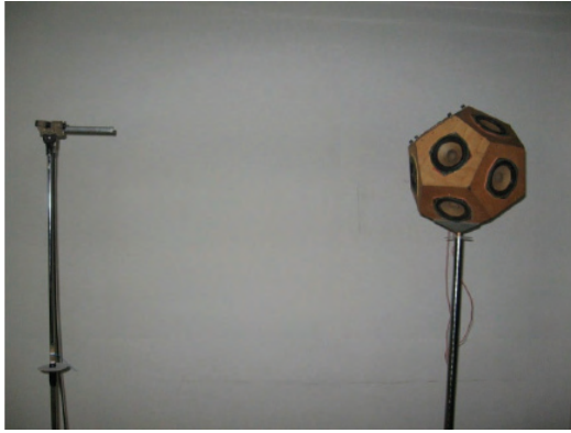
Fig. 4. Setup for directivity measurements of the realized gunshot microphone prototype
