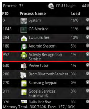
Fig. 5. Processor load by the activity recognition service
