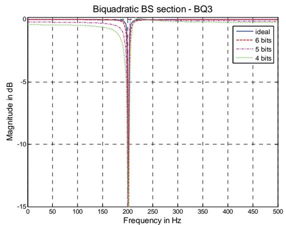
Fig. 4. Sensitivity investigation of low sensitivity structure
