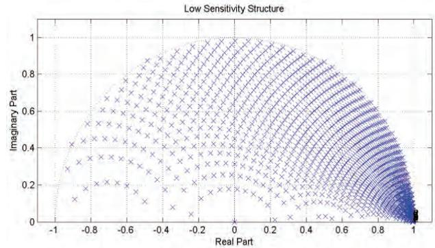
Fig. 2. Possible pole location density of BQ3
