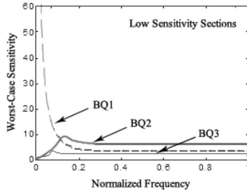
Fig. 3. Worst-case sensitivity investigation of three different low frequency structures
