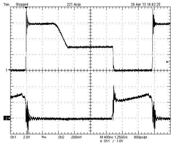
Fig.5. Drain voltage and current waveform at 36V
