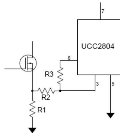
Fig.2. Current sense circuit with bias
