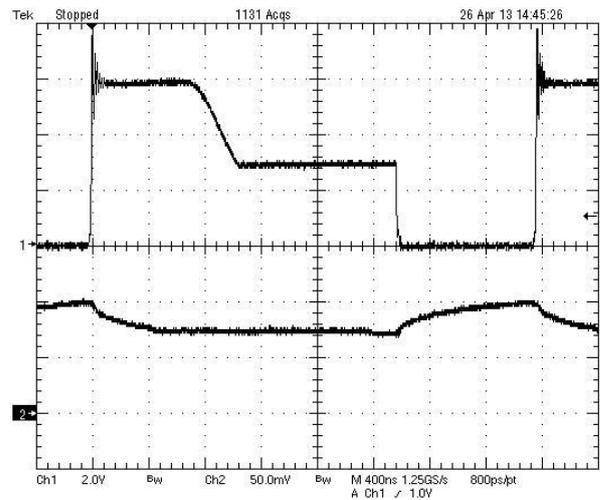
Fig.7. Drain voltage and current waveform (offset) at 24V
