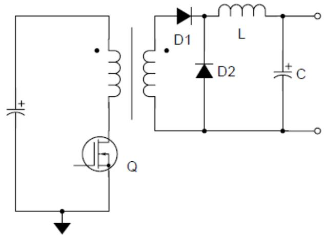
Fig.1. Forward converter
