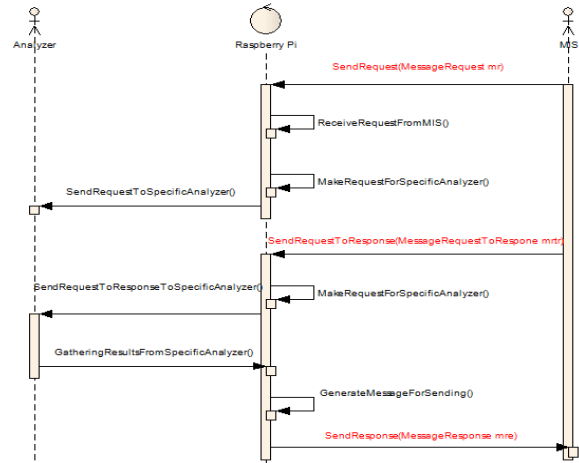
Fig. 4. Sequential diagram of communication between MIS and analyzer.
