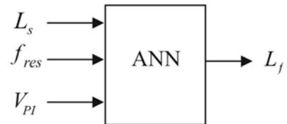
Fig. 2. Proposed inverse electro-mechanical ANN model.
