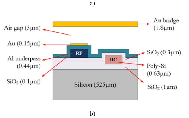
Fig. 1. a) Top-view of the realized switch; b) schematic of the cross-section with 8 layers in FBK technology [11]
