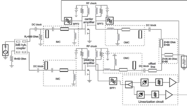
Fig. 1. Schematic diagram of microstrip broadband two-way Doherty amplifier with additional circuit for linearization
