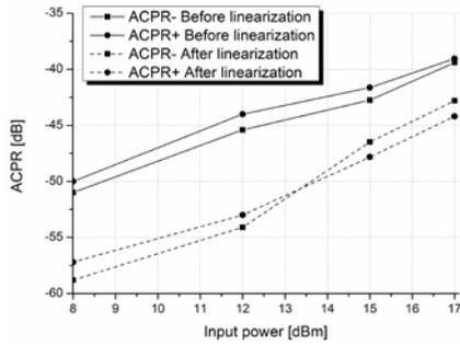
Fig. 4. ACPR before linearization (solid line) and after linearization (dashed line) for WCDMA signal in a range of input power
