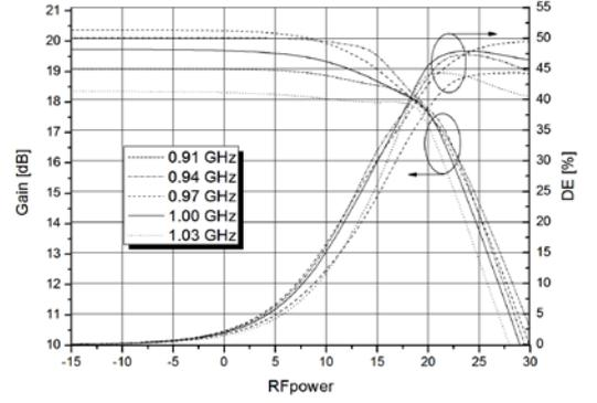
Fig. 2. Gain and DE in terms of one-tone input power at 0.91 GHz, 0.94 GHz, 0.97 GHz, 1 GHz and 1.03 GHz
