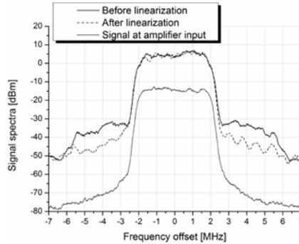
Fig. 5. Signal spectra at input and output of amplifier before (solid line) and after linearization (dashed line) for WCDMA signal at 12 dBm input power
