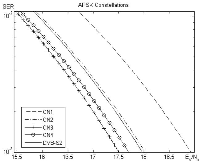
Fig. 3. SER characteristics of 16APSK channels
