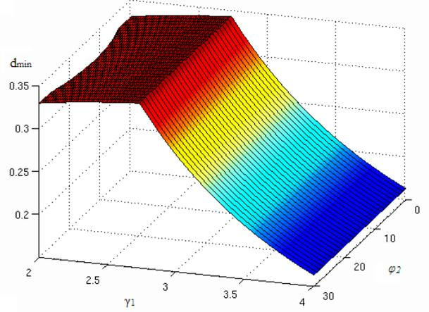
Fig. 2. Minimum Euclidean distances with 4-12APSK in a dependency on  $\gamma_1$  and  $\varphi_2$
