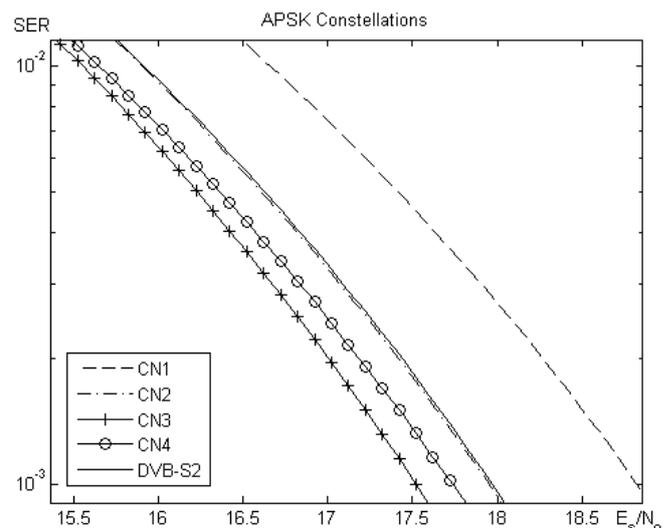
Fig. 5. SER characteristics of 16APSK channels
