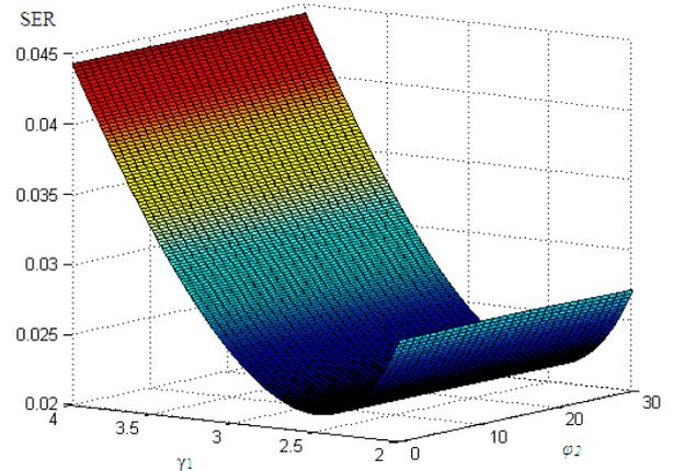
Fig. 4. Dependencies of the symbol error rate for 4-12APSK on the parameters  $\gamma_1$  and  $\varphi_2$
