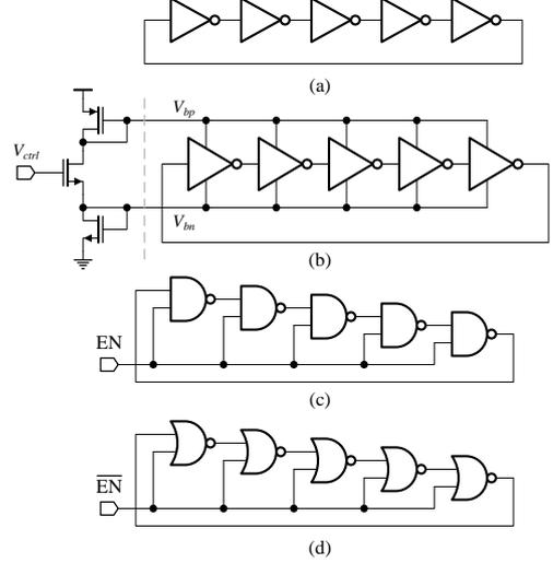
Fig. 3. Logical structures of single ended ring oscillators: (a) basic inverter; (b) current starved; (c) NAND gates; (d) NOR;
