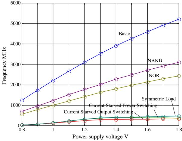
Fig. 5. Operating frequency in terms of power supply voltage
