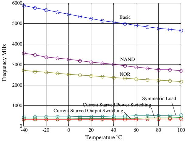
Fig. 6. Operating frequency in terms of temperature
