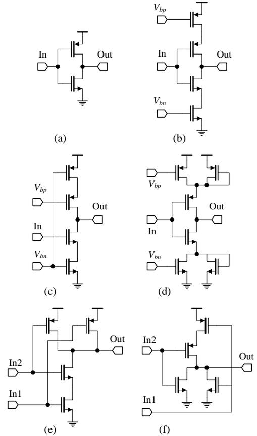
Fig. 4. Electrical schemes of delay elements: (a) basic inverter; (b) current starved with power switching; (c) current starved with output switching; (d) current starved with symmetrical load; (e) NAND gates; (f) NOR;
