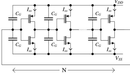
Fig. 2. Conventional voltage controlled ring oscillator
