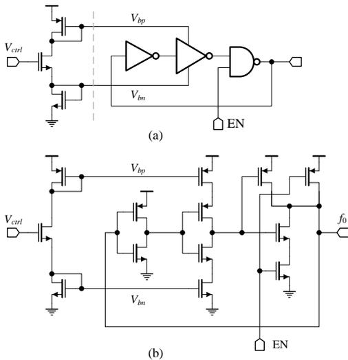
Fig. 8. Three stage single ended start/stop ring oscillator: (a) logical; (b) electrical scheme;
