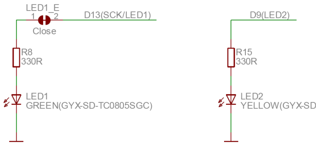
Fig. 2. Light emitting diodes connected to ATmega328P pins 17 (LED1 - digital signal D13) and 17 (LED2 - digital signal D9)
