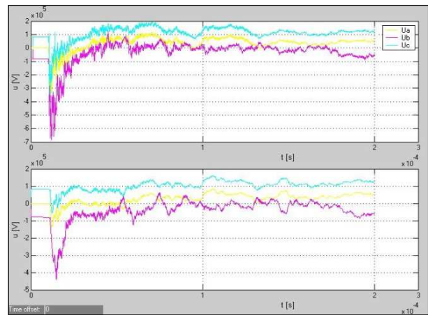
Fig. 7. Voltages in case of lightning stroke on phase B of "Beton" without MOSA in the ES (a) the point of the stroke and (b) on the second transformer terminals
