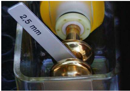
Fig. 5. Calibration of distance between electrodes of 2.5 mm
