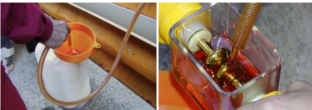
Fig. 6. Realizing oil from device, Filling the container with the sample to measure the oil
