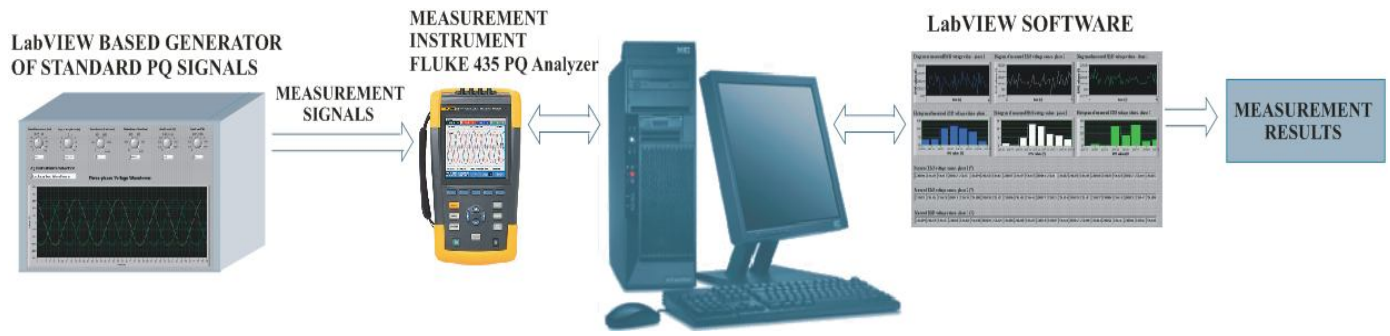
Fig. 1. Block configuration of experimental system for measurement and software processing of standard PQ parameters
