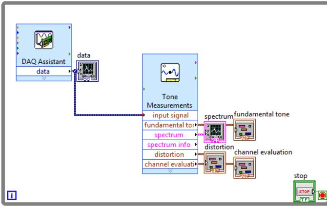
Fig. 6. LabVIEW block diagram.
