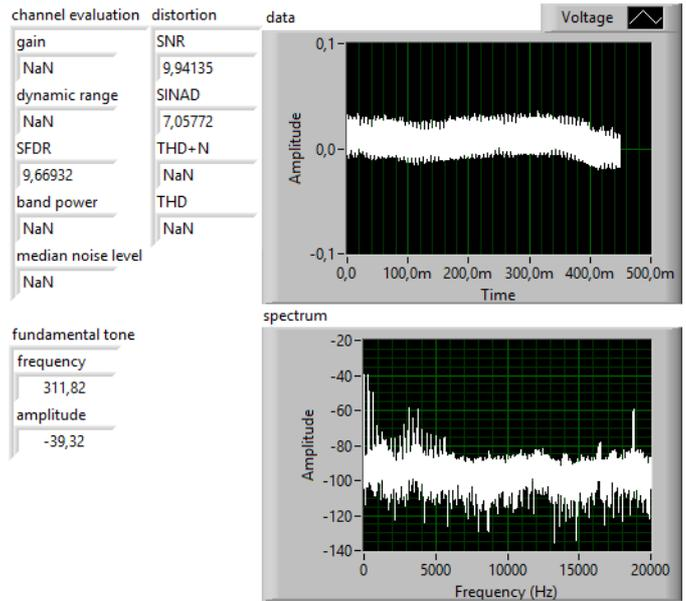
Fig. 1. LabVIEW front panel diagram for fundamental tone measuring in real time: sound „I“ – children's voice
