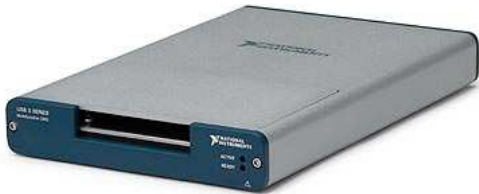
Fig. 2. The external appearance of acquisition cards X series (made by National Instruments)
