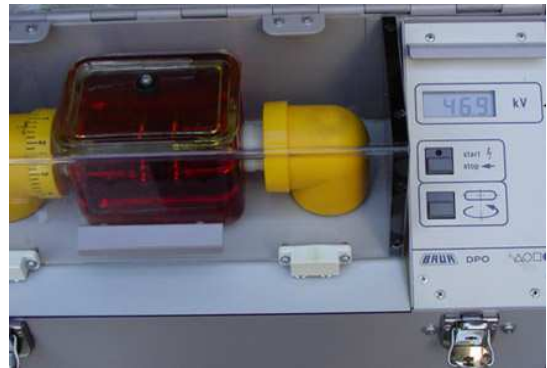
Fig. 7. Measuring of breakdown voltage BDV of the oil
