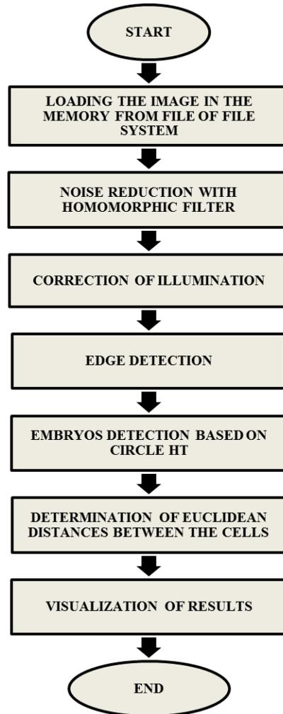
Fig. 1. Block diagram of the basic algorithm
