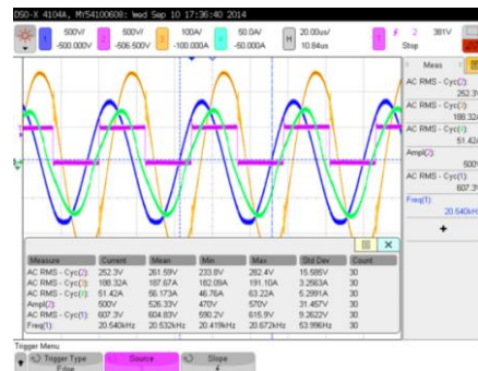
IPT primary current (orange) 188.32A; Matching capacitors voltage CS3-CS10 (blue) 607.3V; IPT secondary current (green) 51.42A; IGBT voltage (pink) 500V at misalignment dx=150mm, power 18.7 kW, frequency 20.54 kHz
