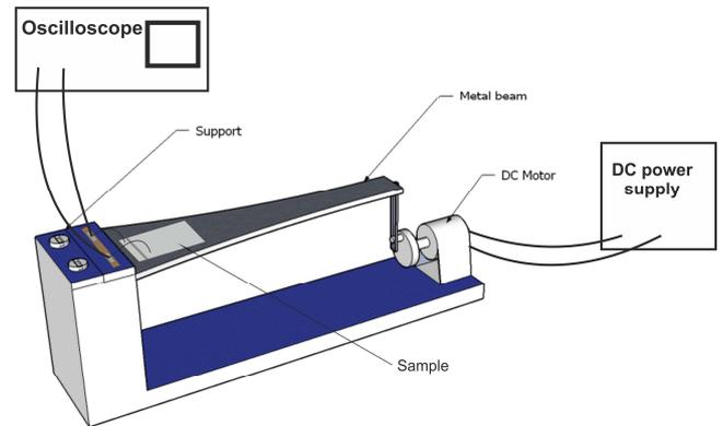
Fig. 3. Experimental setup for dynamic mode measurement of the piezoelectric reaction
