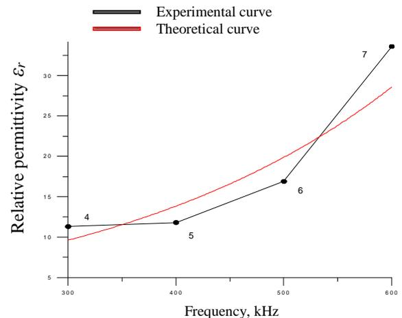
Fig.6. Relative permittivity  $\epsilon_r$  of wet pressed soil from point №2 at a depth of 0.4 m for the sector №2 versus the frequency
