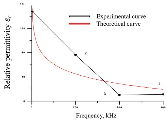
Fig.5. Relative permittivity  $\epsilon_r$  of wet pressed soil from point №2 at a depth of 0.4 m for the sector №1 versus the frequency
