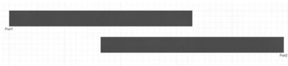
Fig.3 Two coupled resonators with length 32.82mm and width 2.76mm
