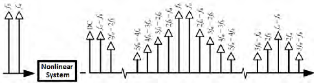
Fig.1. Even and odd-order intermodulation products.
