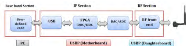
Figure 1 Block diagram of the SDR platform
