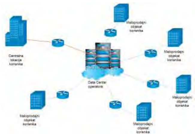
Fig. 1. Managed L3VPN Solution with central location in the operator's Data Center
