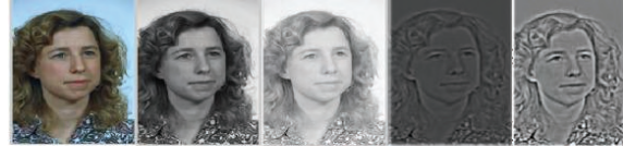
Fig.2. Output of preprocessing original RGB image, Gray image, Gamma correction image, DoG filter image, HE image.
