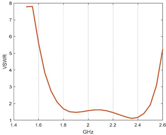
Fig. 5. Simulated VSWR for 1-st frequency band
