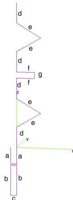
Fig.4. Proposed design of super J-pole fractal antenna
