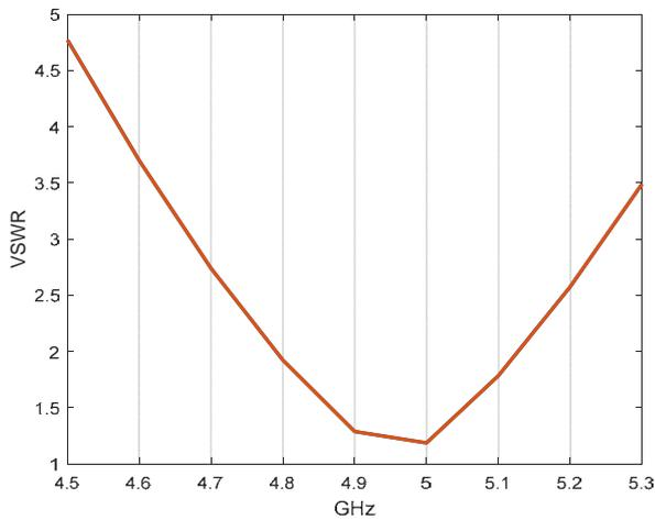
Fig. 6. Simulated VSWR for 2-nd frequency band
