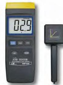
Fig. 1. Measuring device Lutron EMF-828 with separate probe
