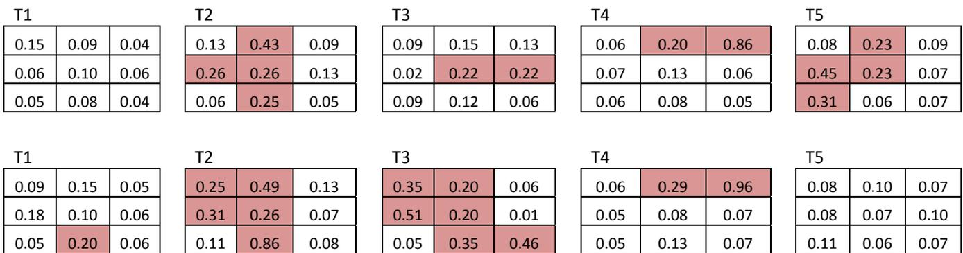
Fig. 3. Magnetic field measurement level (Top position represents measurement at the top of the tablet (touchscreen display area). Bottom position represents measurement at the bottom areas of the tablet. Colored fields represent the areas with higher emission than it is allowed)
