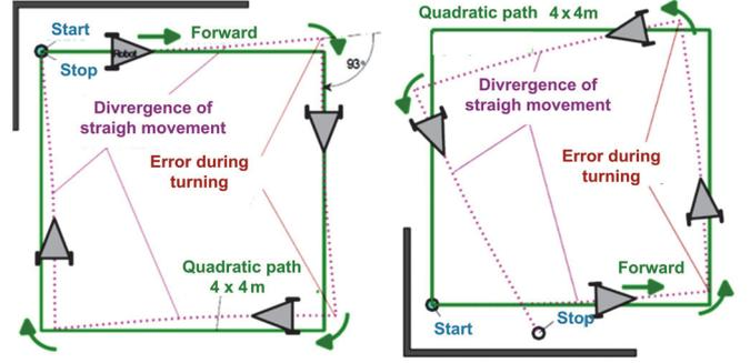
Fig. 2. Robot movement in bidirectional test on quadratic path
