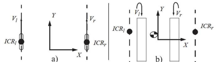
Fig. 1. Position of point of rotation  $ICR_l$  and  $ICR_r$  for wheeled robot (a) and for tracked robot (b) [3]
