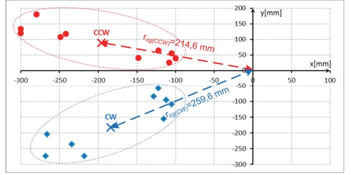
Fig. 3. Odometry errors in bidirectional test prior correction
