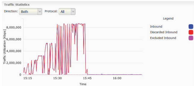
Fig. 4. Input traffic to Customer1 during attack
