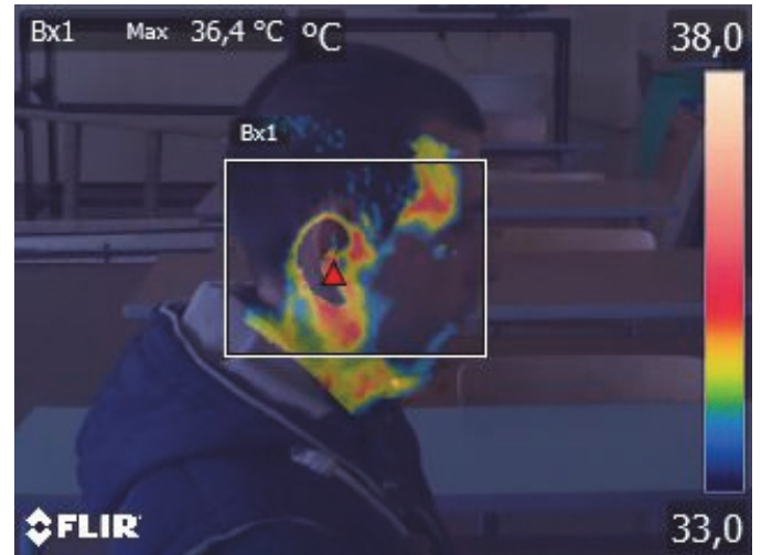
Fig. 4. Temperature t [°C] on the head profile plane for Object#2 in current time \tau=40 min
