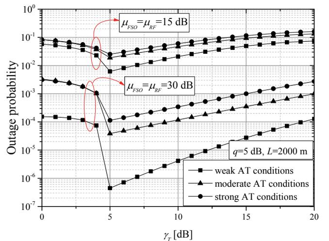
Fig. 4. Outage probability versus the switching threshold in various atmospheric turbulence conditions
