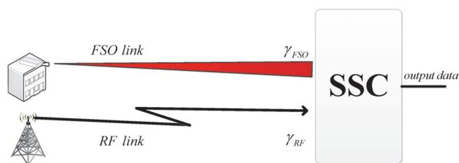
Fig. 1. System model of hybrid RF/FSO system
