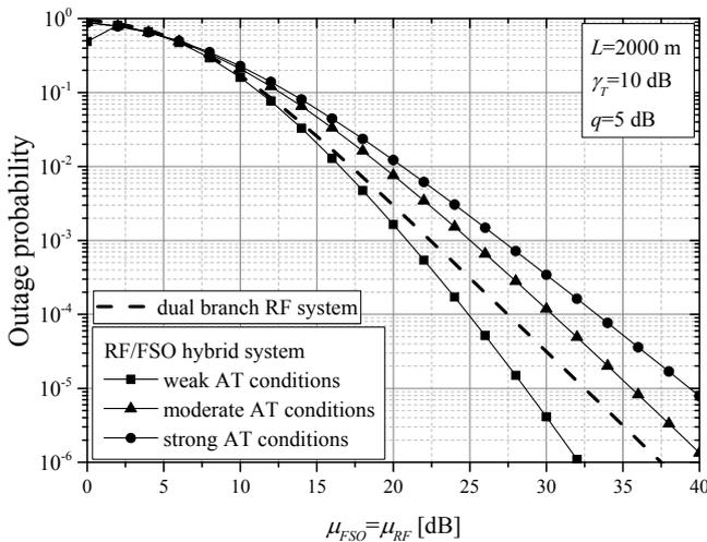
Fig. 2. Outage probability versus  $\mu_{FSO}=\mu_{RF}$  for hybrid RF/FSO and dual branch RF system
