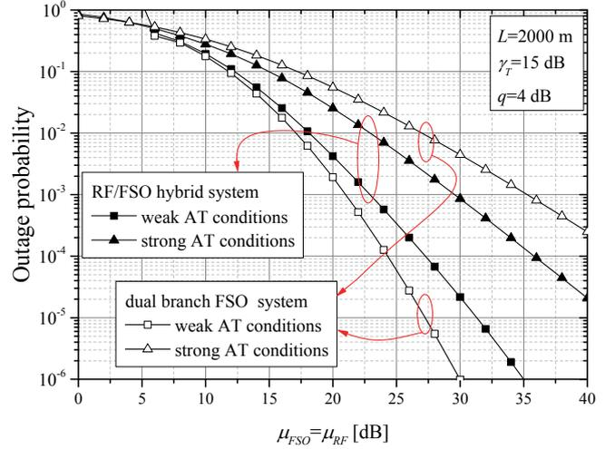
Fig. 3. Outage probability versus  $\mu_{FSO}=\mu_{RF}$  for hybrid RF/FSO and dual branch FSO system
