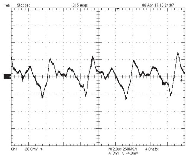
Fig. 6. Output ripple at full load
