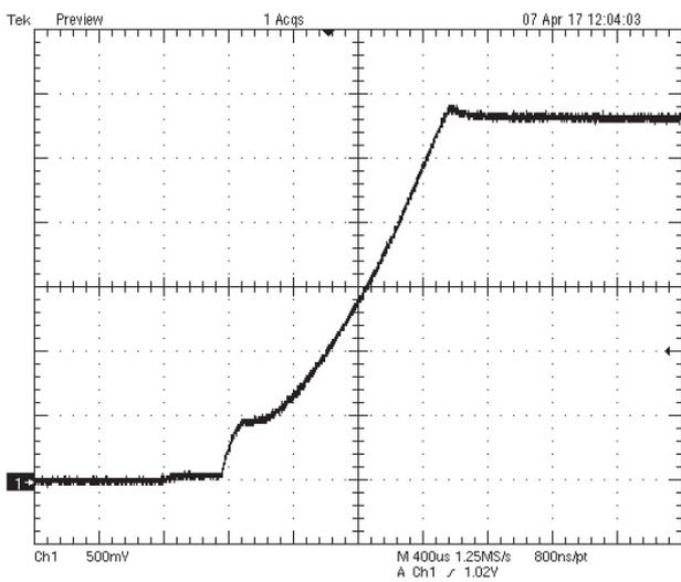
Fig. 9. Output voltage rise into full load at turn on
