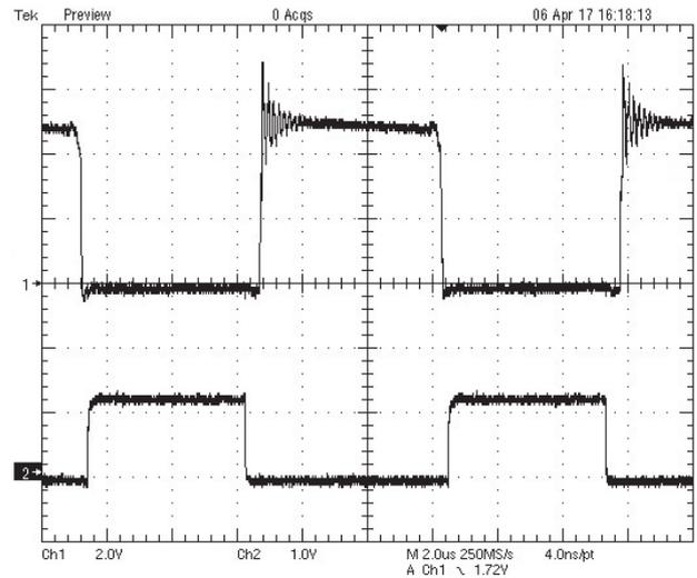
Fig. 5. Drain and gate voltage of FET Q<sub>4</sub>
