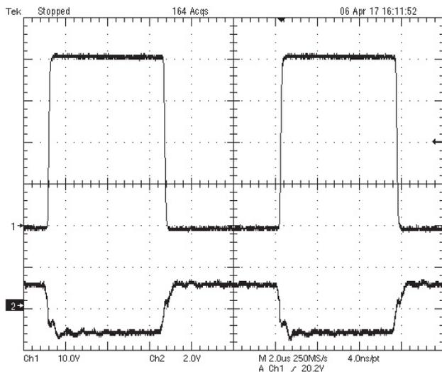
Fig. 3. Drain and gate voltage of low side FET Q<sub>2</sub>
