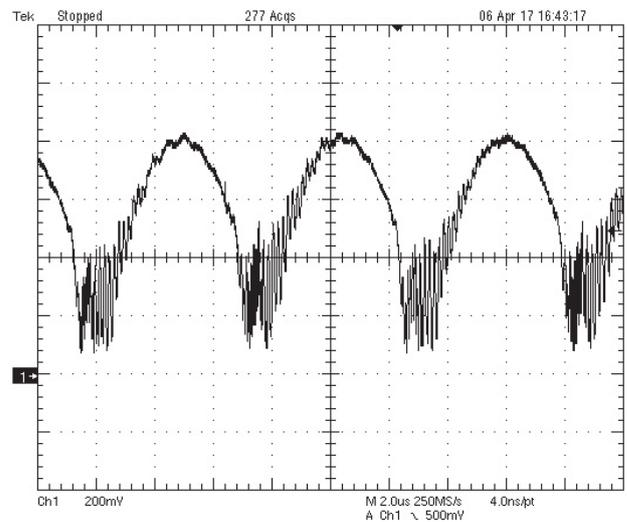
Fig. 7. Primary current (rectified at current sense)
