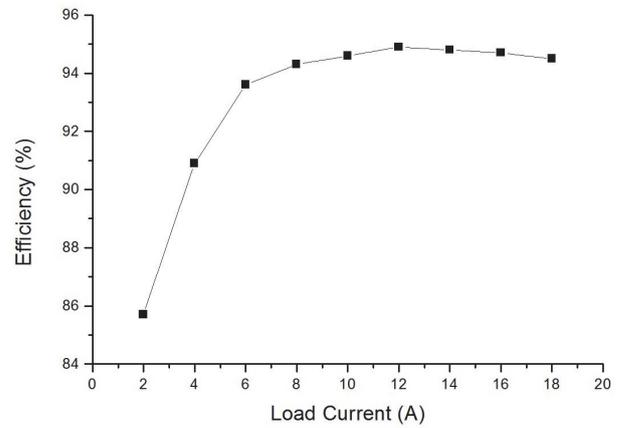
Fig. 12. Efficiency vs. load current
