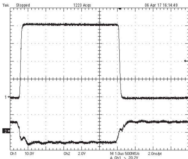
Fig. 4. Drain and gate voltage of low side FET Q<sub>2</sub> (zoomed in)
