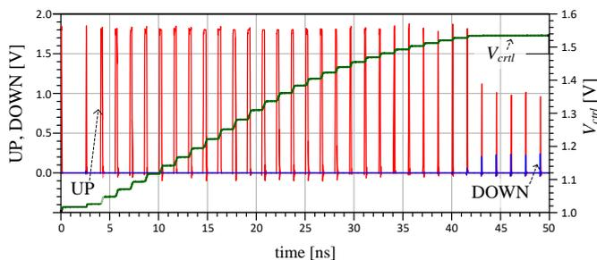
Fig. 8. Transient response of DLL-CLK Skew Compes
