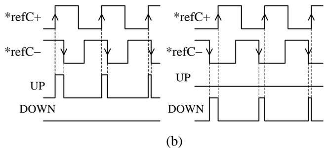
Fig. 3. PD transistor schematic (a), waveforms of PD (b)
