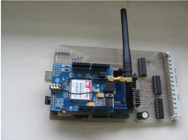
Fig. 5. Arduino Mega interface board with the GSM module attached (Arduino SIM800C Module)
