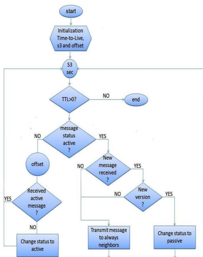
Figure 5. Block diagram of Message transmission algorithm
