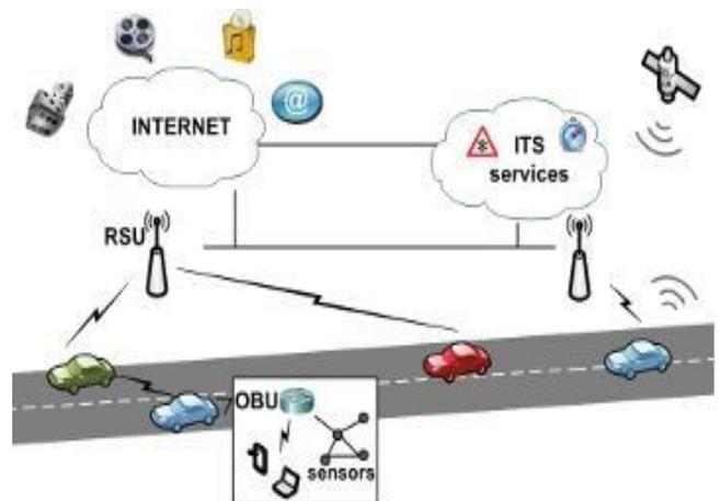
Figure 1. Network Architecture and communication types in VANET
