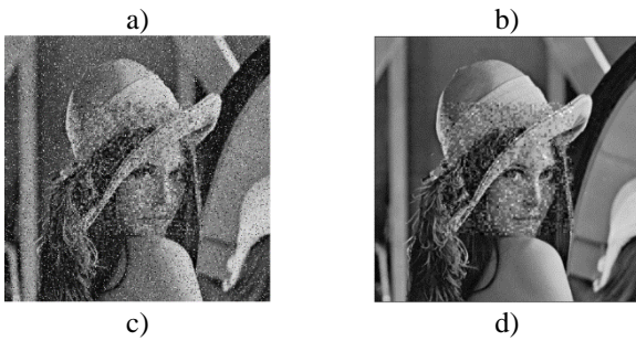
Fig. 3. Watermarked image Lena with k = 4 and p = 10 : a) noised, b) filtered, c) recovered from noised image, d) recovered from filtered image.
