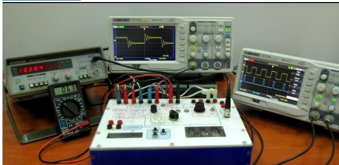
Fig. 2. The proposed kit in use (at the moment of taking the photo, the variable resistor in the loop filter is not adjusted to its optimal value.
