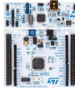
Fig. 2. Nucleo L476RGT6 development board
