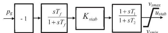
From the stabilizer is required damping of oscillations that are of a local character and an inter-area character. Depending on a type of oscillation, the stabilizer performs phase compensation in a certain frequency range. The phase characteristic to be compensated, changes with the change in the state of the system, so the setting of the stabilizer for one condition does not mean a satisfactory setup for another state of the system.
