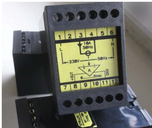
Fig. 2. The transducer's front panel and housing
