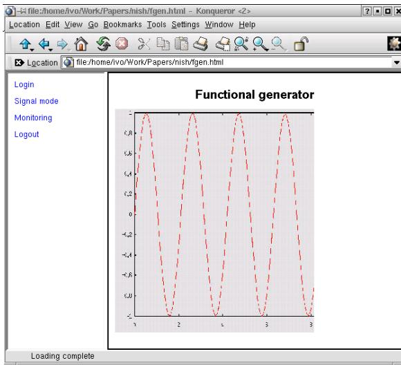
Fig. 3. An example of web monitoring of the generated signal. Parameters: sinusoidal waveform, phase= $0^\circ$ ,  $U_{out} = 1V$  and  $f_{out} = 0.5Hz$
