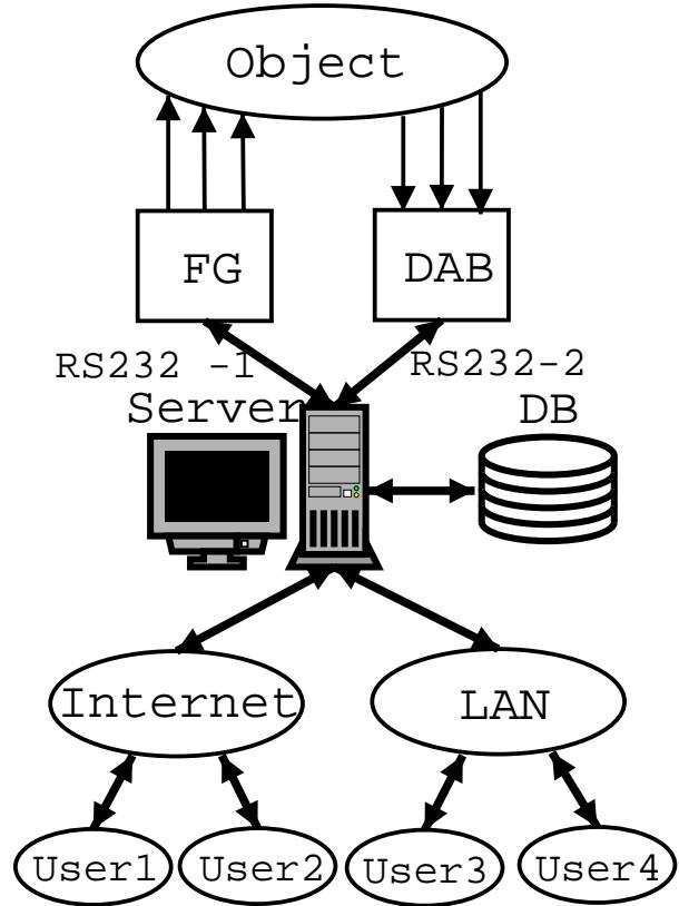
Fig. 1. Computer-system architecture of functional generator controlled by computer network.
