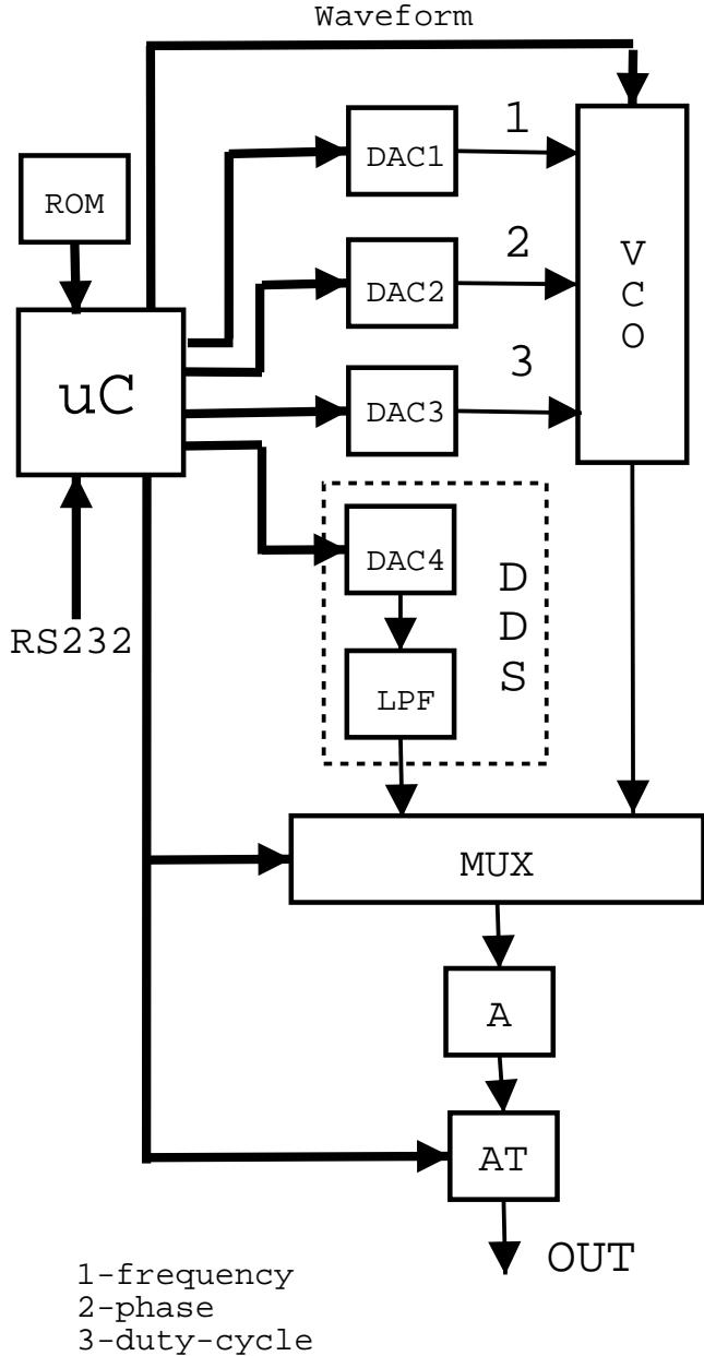
Fig. 5. Block diagram of the functional generator board.
