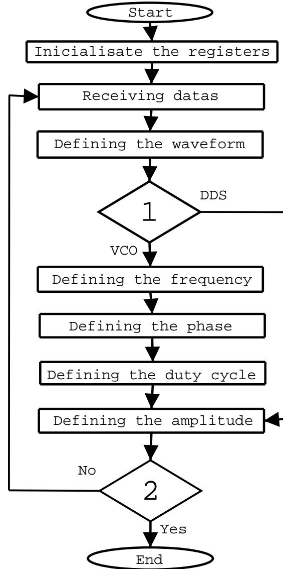
Fig. 6. Algorithm of the functional generator board.
