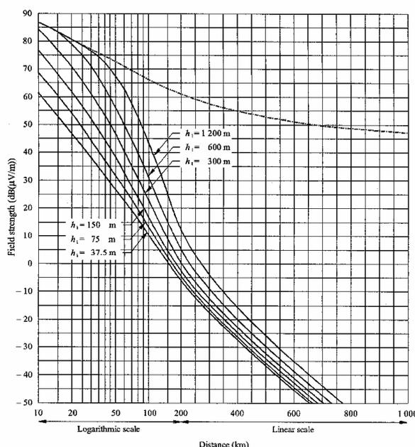
Fig. 1. Field strength (dB(μV/m)) for half wave dipole, which radiates 1 kW e.r.p. [1], land, 50% of the time, 50% of locations, frequency 450-1000 MHz
