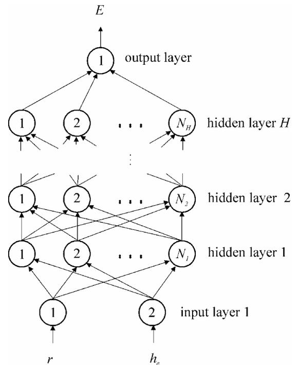
Fig. 2. Neural model architecture used for prediction of the electric field level  $E$  as a function of effective height  $h_e$  and distance between receivers  $r$
