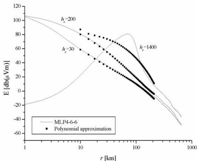
Fig.5. Comparing output curves of MLP model to values obtained by polynomial approximation application for the cases of  $h_e=30$  m and  $h_e=1400$  m that are not belonging to a range of training neural models.
