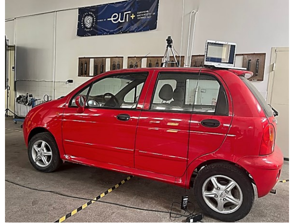
Figure 1. Experimental setup showing the stationary idling vehicle and the position of the particulate matter sensor in the enclosed hall
